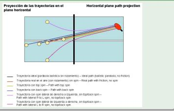
Contact with a surface Trajectory in the air. Magnus effect
