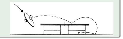
Contact with a surface Trajectory in the air. Magnus effect
