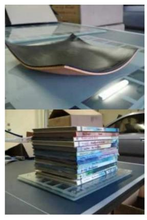
The rubber is already much bigger at this stage. Important Note: Using this many layers of glue can put quite a bit of strain on rubbers, so if you're not confident that the topsheet and sponge are glued together well, use less layers, or at least enough layers to get a decent dome.
